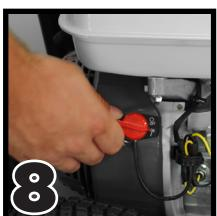
Switch engine to "on".
