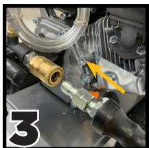
Connect high pressure hose to the pump outlet.
